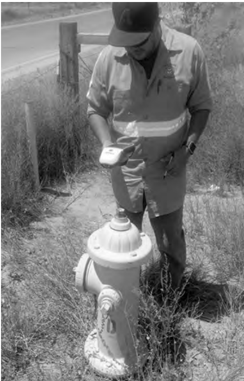
Mr. Kevin Jojola downloading information on the location of a fire hydrant into a GPS device.
